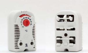
The TTEC series are thermostat controllers used to regulate the temperature inside industrial control panels or cabinets and control cabinet accessories. The TTEC series, bimetallic thermostats, control fans, heaters, and switch loads. TTEC-100 and TTEC-200 are identical except the TTEC-100 is Normally Closed which opens at temperature rise, the TTEC-200 is Normally Open which closes at temperature rise. Both are available in Fahrenheit or Celsius
